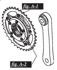
Check the button-head bolts on the main body for tightness (fig. A-2)
